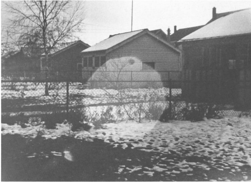
Figure 6.17. An in-focus diaphragm image on the film (enlarged from a 16mm frame).
