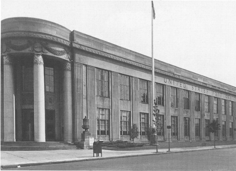
Figure 1.5. The effect of tilting a camera sideways.
