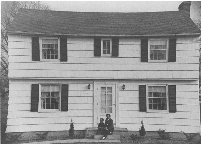
Figure 2.23. A photograph taken with a poorly designed telephoto lens, showing pinchusion distortion.
