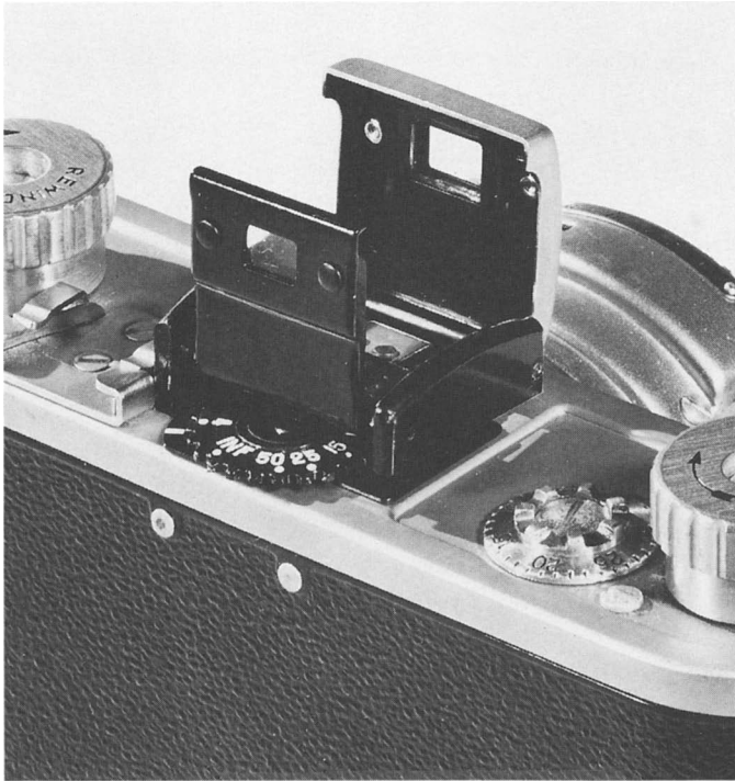
Figure 12.8. Viewfinder equipped with means to correct line-of-sight parallax.
