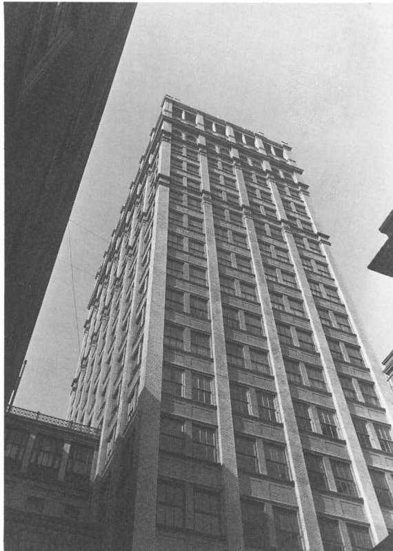
Figure 1.3. Keystone distortion resulting from an upward tilt of the camera.
